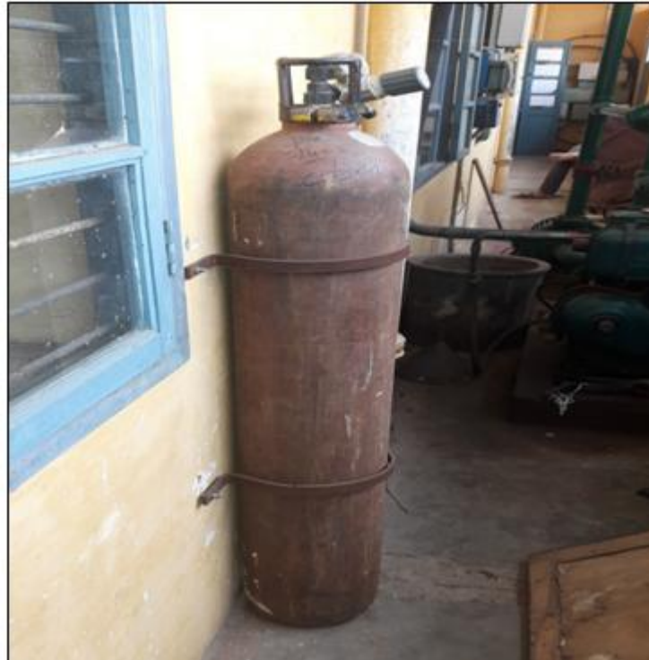
Fig 4.2 Photographic view of Hydrogen cylinder
